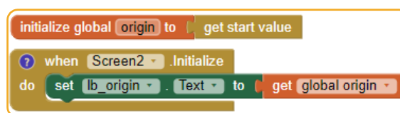
Fig. 20 Code that stores the value sent from Screen1 in a variable and shows its in a label at Screen2
