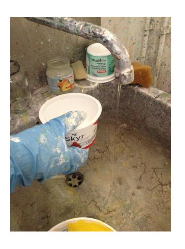
Add a little bit of water (20-30% of the amount of the varnish) into the mixing cup to make the varnish thinner.
