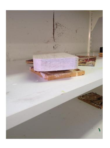
Put the work piece to dry in to a safe place on top of the bars. Check the drying times from the package of the varnish you used. Sand the surface and possible pouring marks with a smooth sand paper before applying the second coat of varnish. You can apply a third coat of varnish if you want to, but this time you do not have to sand the whole surface.
