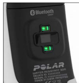
Figure 3. Optical measurement at the back of the wrist unit: two green LEDs as light emitters and a square photodiode as the light detector between the LEDs.
