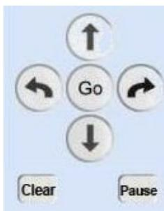
In a programming language, such as Logo, a program is a sequence of commands that are executed in the order specified. With the Pro-Bot, like the multi-award winning Bee-Bot®, a simple program can be developed using only the four arrow keys. Surprisingly complex and extended sequences can be created without requiring any other keys.
