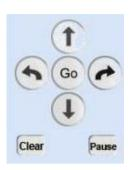
In a programming language, such as Logo, a program is a sequence of commands that are executed in the order specified. With the Pro-Bot, like the multi-award winning Bee-Bot<sup>®</sup>, a simple program can be developed using only the four arrow keys. Surprisingly complex and extended sequences can be created without requiring any other keys.
