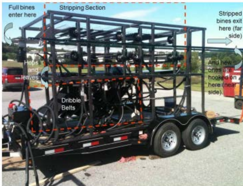
Figur 7. Mobil, traktordriven plockmaskin, UVM Mobile Hops Harvester, utvecklad vid University of Vermont Extension (Mobile Hop harvester, 2014).
