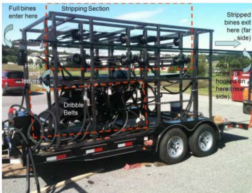
Figur 19. Mobil, traktordriven plockmaskin, UVM Mobile Hops Harvester utvecklad vid University of Vermont Extension. (Mobile Hop harvester, 2014).
